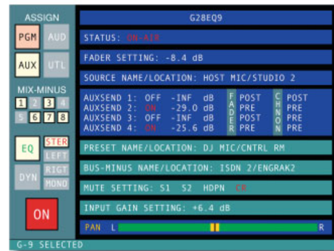
Press an input SET button and detailed information pops up on the above screen, showing complete channel status.
