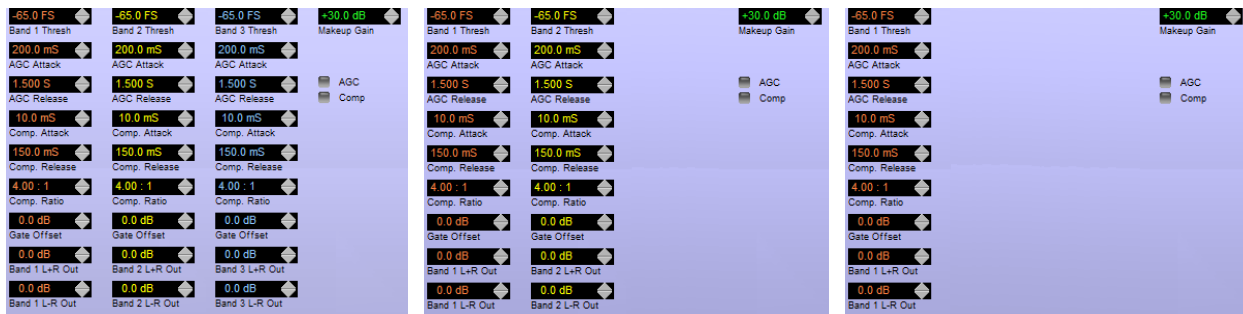
Comparison of AGC controls visible in 3 band mode (left), 2 band mode (center), and broadband mode (right)
